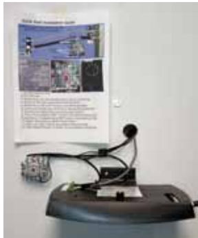
Photo: Correct routing of cables to avoid radio interference with base antennae.
